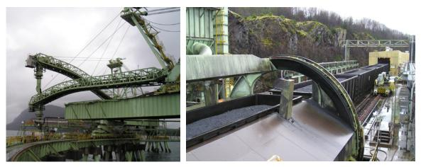
Continuous rotary rail car dumper and coal transfer at Prince Rupert
