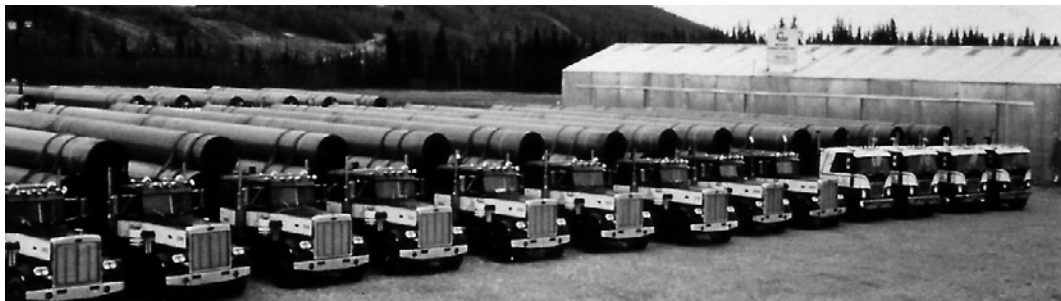
Alyeska Project 48 inch diameter/80 foot length pipe haul by truck from Fairbanks
